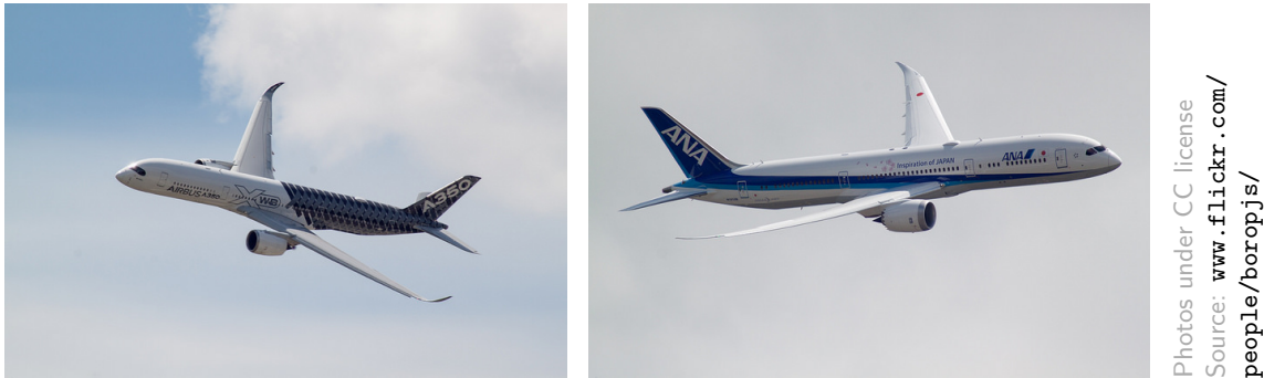
Figure 1.1: Photos of Airbus A350 (left) and Boeing Dreamliner 787 (right). Both airplanes have higher wing aspect ratio and exhibit larger structural flexibility than previous generations.
